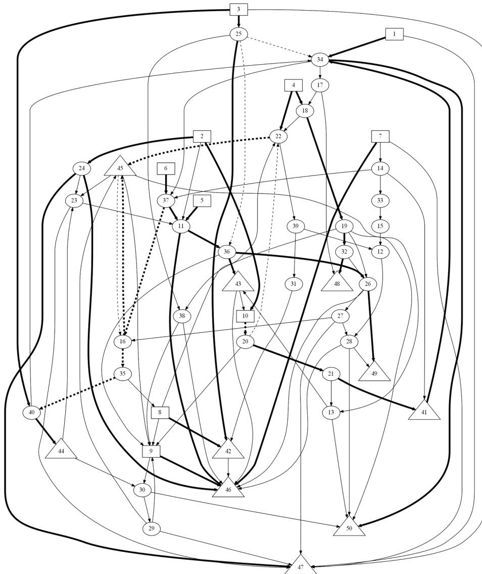
FIG. 5.3. Diagram showing decision-making at time 0 under the heterogeneous-prior setup. Rectangles represent supply nodes; triangles represent demand nodes; ovals represent transshipment nodes. Lines in bold indicate edges with nonzero flow according to x^*(c^0) . Dashed lines indicate edges with high KG factors.
